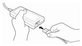
Figure 3-1 Connecting the power cord to the AC adaptor
